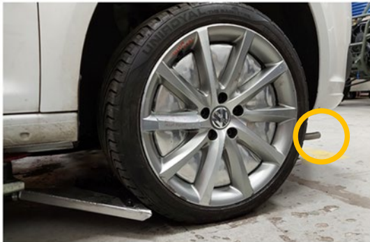
Tyre sample duct fitted behind wheel
