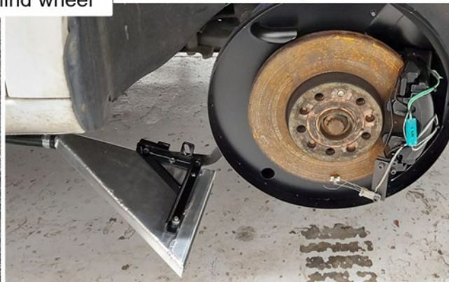
Wheel removed showing mounting of tyre sample duct, and rear of brake enclosure
