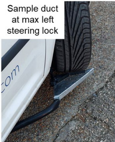
Tyre sample duct fitted behind wheel
